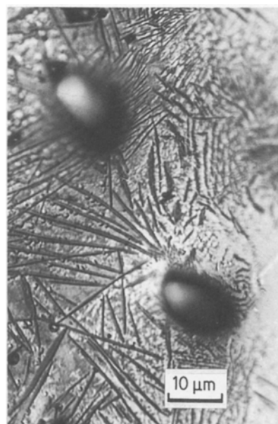
Figure 3 Growth of plates around SiC particle.
